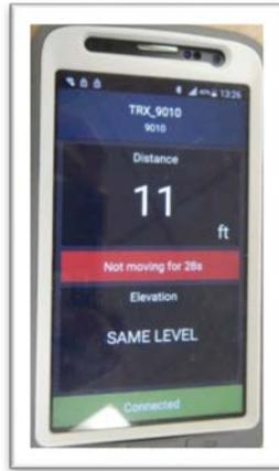
Figure 2 - Handheld display carried with a paired TRX proximity unit by the team lead or incident commander.
