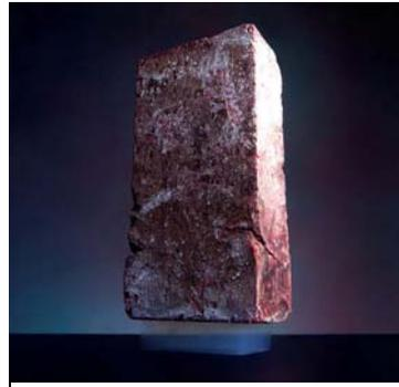
Figure 3.2. Aerogel Supporting a Brick.
