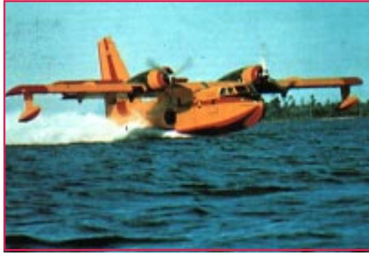
**Figure 2**—A Canadian CL-215 scooping water from a lake. This aircraft, with its 1,400-gallon (5,300-L) water-scooping and optional foam injection capabilities, is an excellent tool for firefighting support in the Lake States. Photo: Minnesota Department of Natural Resources, Grand Rapids, MN, 1997.
