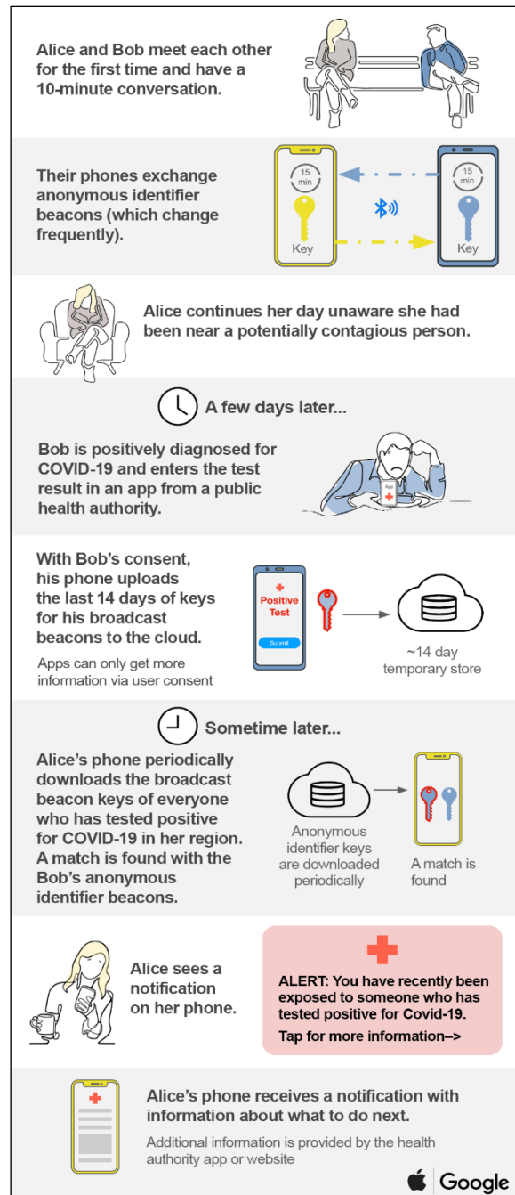
Figure 1. Apple-Google Digital Exposure Notification Using Bluetooth
