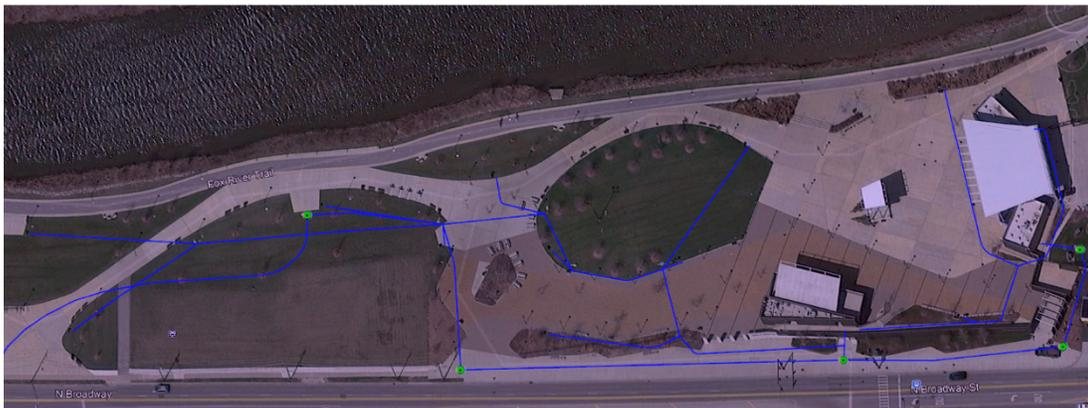
Figure 1. Fiber Optic Network at RiverEdge Park
