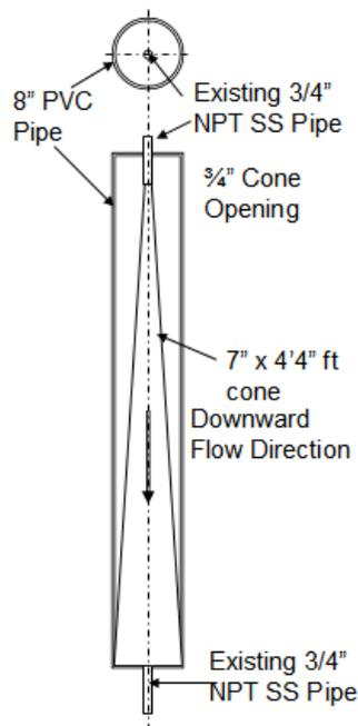
**Figure 3: Cone diffuser used for ozone concentration with national pipe thread taper (NPT) stainless steel (SS) pipe.**
