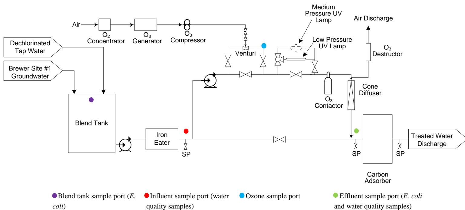
**Figure 1: Schematic diagram of the pilot-scale AOP system with sampling ports.**
