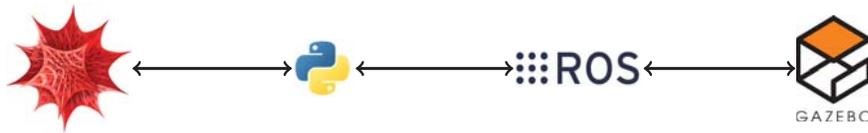
Figure 18: A diagram of the control structure. Differential equations are solved in Wolfram Mathematica using Euler’s method. ROS receives desired data using Python and transmits it to simulated robots in Gazebo. Feedback is relayed back to Mathematica through ROS using Python.
