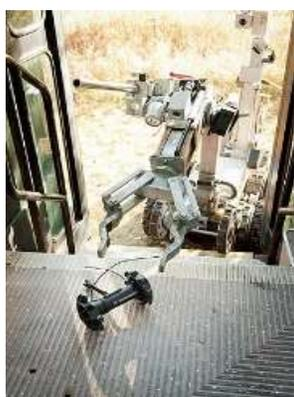
**Figure 4. Bomb disposal robot dropping a throwable robot onto a bus**
