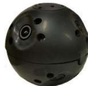
**Figure 5. Spherical scouting robot**
