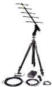
**Figure 3. Command monitoring station**
