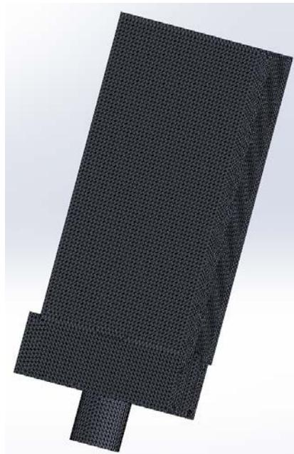
**Fig. 7 Mesh with 0.01-inch element size**
