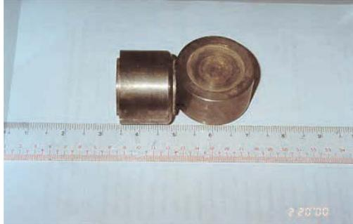
Figure 3. Housing unit. The left portion is hollow and housed the Cobalt-60 source.
