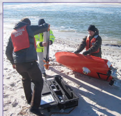
U.S. Geological Survey scientists prepare an acoustic doppler current profiler to measure water velocity profiles in a new inlet formed during Hurricane Sandy on Fire Island, New York.
