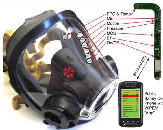
The flexible WiPEM unit is mounted inside the SCBA mask. The curved piece rests against the firefighter's temple.
