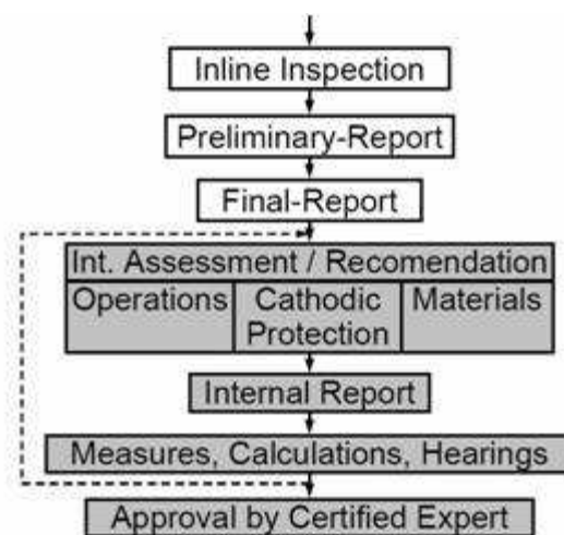
Figure 2: Processing of Pig Run Results at E.ON Ruhrgas
