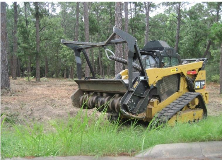
A close up look at the skid steer tractor with its mulching unit
