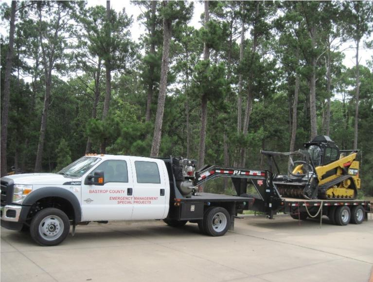
One of four units purchased for the project. This truck was equipped with a 100 gallon diesel tank on its bed, a flatbed trailer and a skid steer tractor. (Photo by: Bonnie Hanchett)
