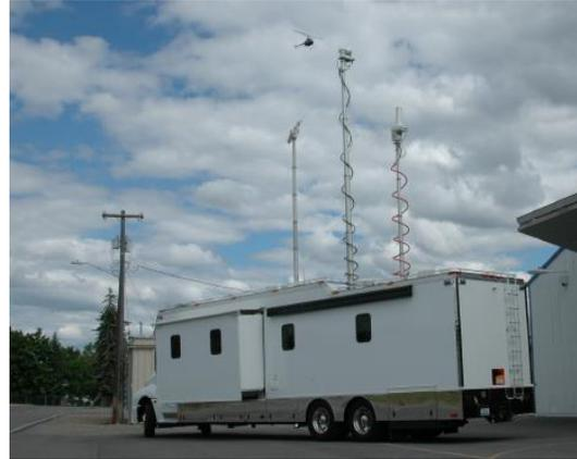
Mobile communications vehicle used to provide shelter and operational space for coordinated on-site incident response.
