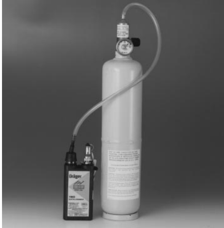
Figure 13. CO Data Logger
