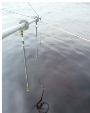
Figure 2. Dispersant spray arm
