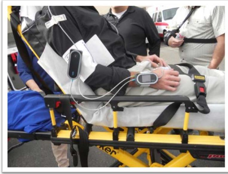
**Figure 6 - ViSi Mobile worn while patient is on a stretcher**
