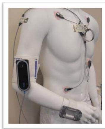
Figure 4 - ViSi Mobile emplaced on a mannequin
