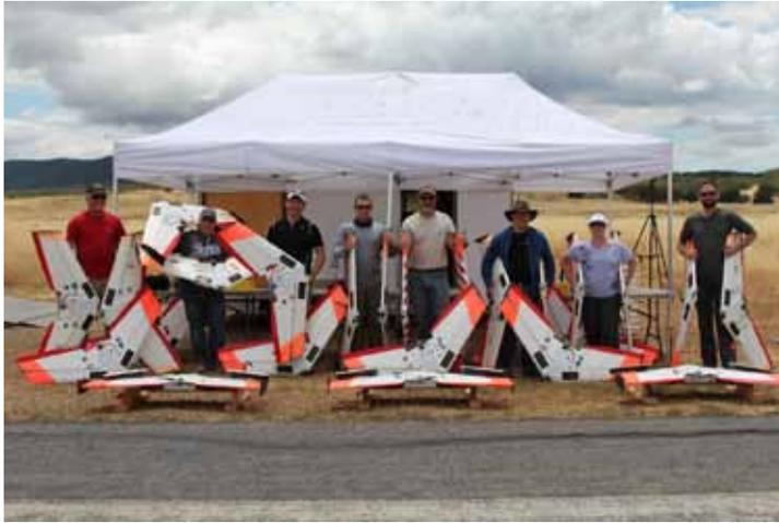
On the afternoon of May 15th, the team launched 20 lightweight autonomous aircraft using a bungee-driven catapult launcher. The aircraft used are flying wings made of Styrofoam and outfitted with hobby-grade components. Each plane is also equipped with an autopilot that can perform waypoint-based navigation and a secondary computer that communicates with other aircraft as well as ground systems, and coordinates cooperative flight.
