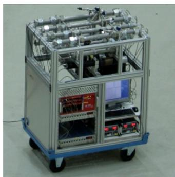
**Figure 4.** Array of seven  $^4\text{He}$  detector modules.
