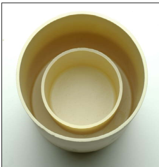
Figure 3.A Crucible for Electrorefining Plutonium
