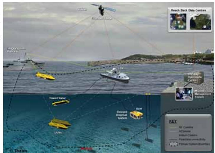
Figure 1: Representation of MMCM concept (Courtesy of Thales)
