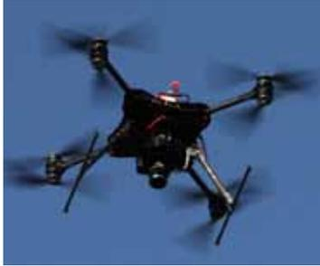
At the JIFX, the sUAS platform used for the Pixelteq SpectroCam™ multispectral camera was an eight-engine multicopter controlled with a 3DR open-source Pixhawk flight control computer as found in many commercial systems. The system consumed roughly 18,000 watts of power to manage both the flight control, sensor operations
