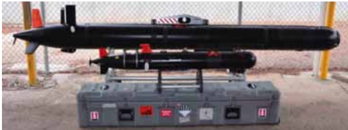
Figure 1: Mk 18 Mod 1 and Mod 2 UUVs. (Image courtesy of Space and Naval Warfare System Center, Pacific.)
