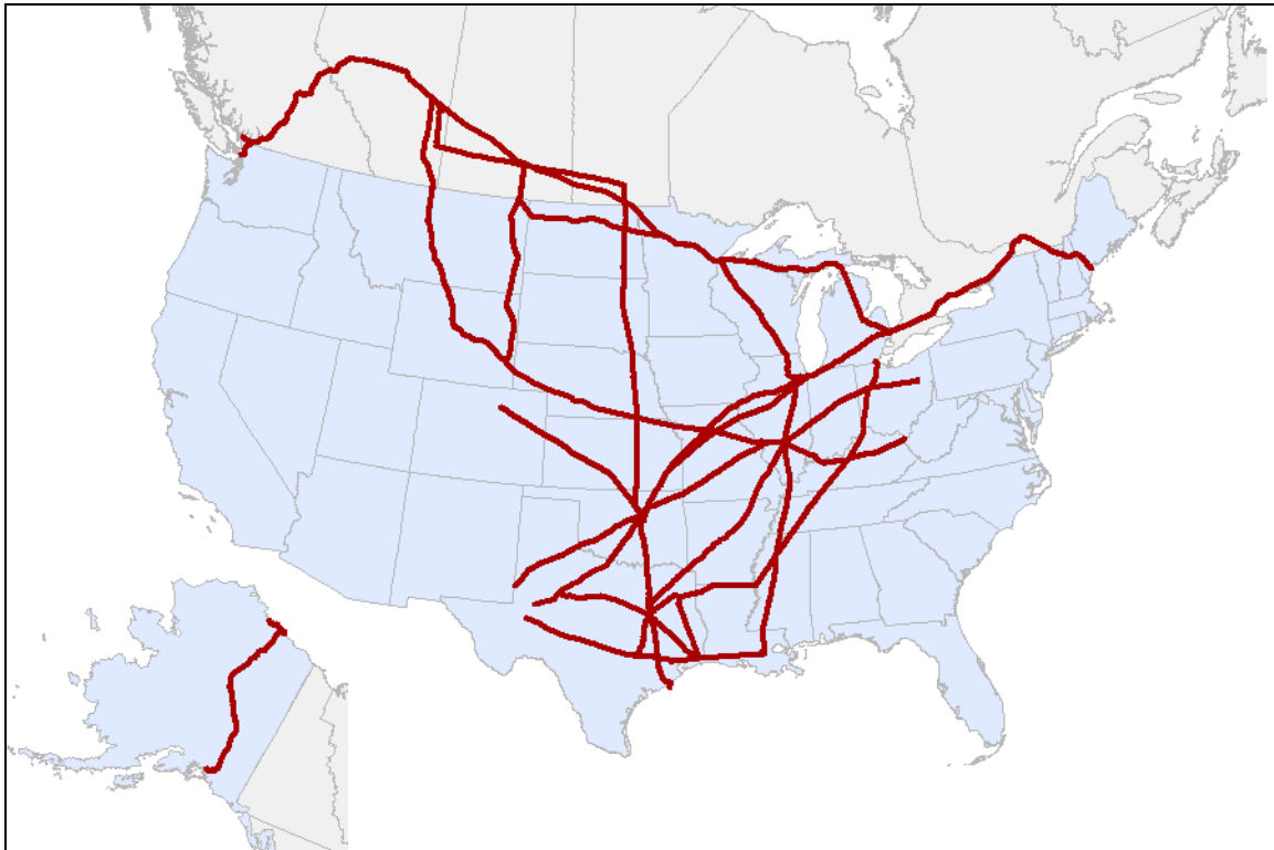
Figure 5. Major U.S. and Canadian Crude Oil Pipelines
