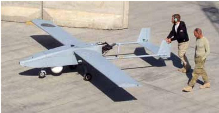
Sandia's Copperhead — a highly modified MiniSAR system mounted on unmanned aerial vehicles (UAVs) — has been uncovering IEDs in Afghanistan and Iraq since 2009. Now, Sandia is transferring the technology to the U.S. Army.
