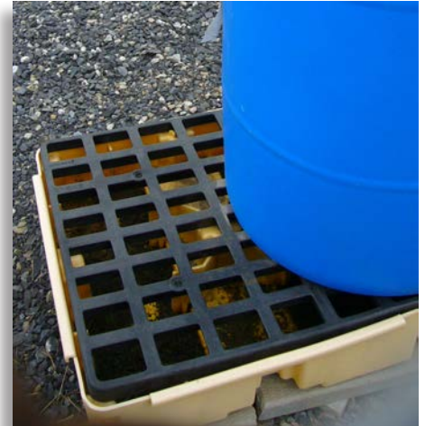
This yellow polyethylene containment pallet with the black plastic deck is used for the outdoor storage of a corrosive hazardous liquid.
