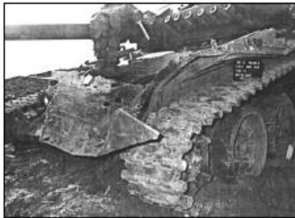
Figure 3. Photograph from the 1988 Soviet Artillery Effects Study showing the results of one 155mm high explosive round
