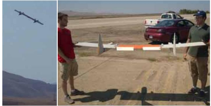
*The 8 foot Chimera UAV was constructed with 3D printed cambered flaps, wing ribs, and a three-axis gimbled camera system. Image Credit: NASA Ames)*
