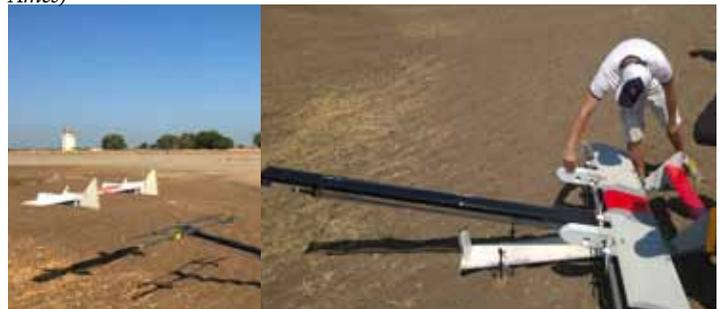
*An adjustable bungee-powered launch system was designed and constructed to enable launch of a three-fuselage wide configuration. Shown above are the twin-fuselage Chimera and the Alicanto UAVs. Image Credit: NASA Ames)*
