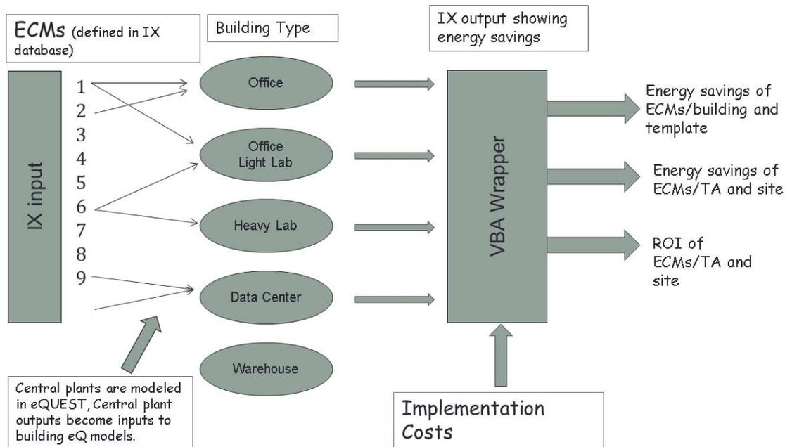
**Figure 1. Schematic of IX Model**
