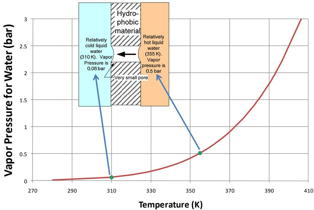
Figure A-1: Schematic of Membrane Distillation Unit Operation
