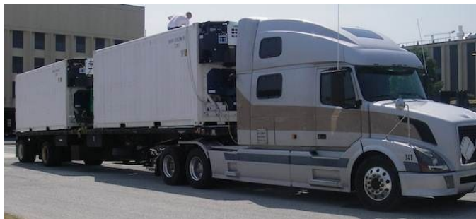
Figure 6. The SuperMISTI system mounted on a 48-ft trailer for testing prior to deployment to the Manta technology demonstration.
