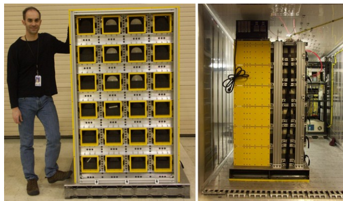
Figure 1. Pallet-mounted HPGe array. (left) Front view of array. (right) Side view of array installed in ISO container.
