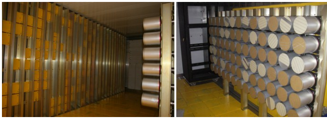
Figure 2. (Left) 12 \times 27 lead coded aperture mounted to ISO container wall. (Right) 6 \times 13 array of NaI detectors on opposite side of ISO container.
