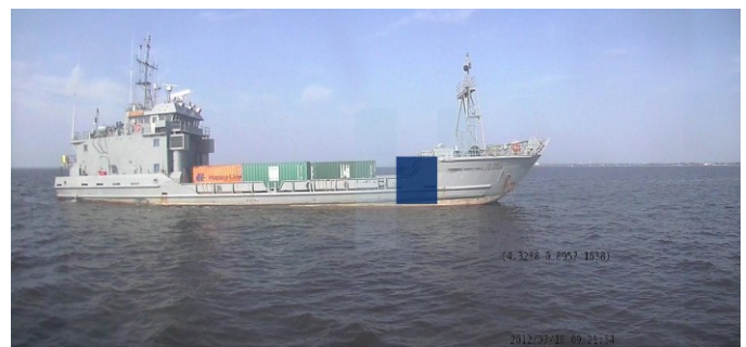
Figure 4. Reconstructed radiation source position image for a gamma-ray source located on a ship. The dark blue square indicates the source location.
