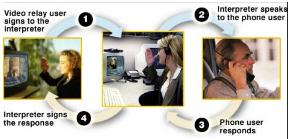
Figure 1. How Video Relay Service Works
