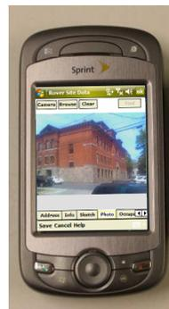
Left: Building vulnerability data are collected in the field with ROVER on a smartphone.
