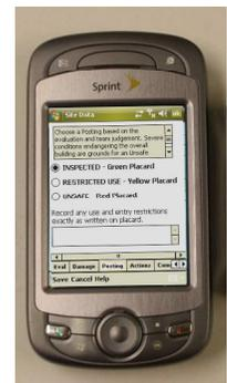
Right: ROVER is used for safety tagging by inspectors after an earthquake.
