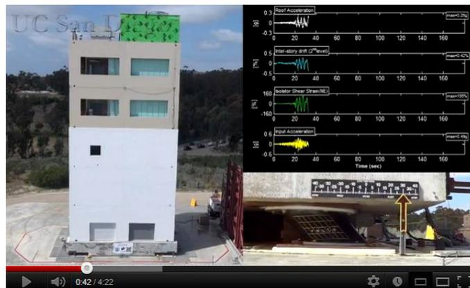
Excerpt from [video on BNCS test](#) conducted in April 2012. Left side shows test building on UCSD shake table. Upper right shows instruments tracking motion parameters captured by building sensors. Lower right shows base isolator flexing under the building (vertical arrow measures lateral movements). Courtesy of BNCS Project Core Team.
