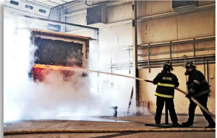
The hose stream test is intended to evaluate fire assemblies' ability to remain intact. (Photo/Architectural Testing, York, Pennsylvania)
