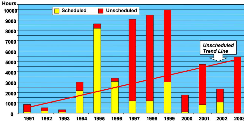
Figure 5: Upper Mississippi River lock unavailability time due to scheduled or unscheduled maintenance or hardware malfunction.
