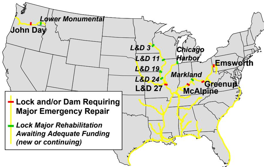
Figure 7: Major locks and dams requiring emergency repairs, November 2002 through August 2004, and pending major rehabilitations.
