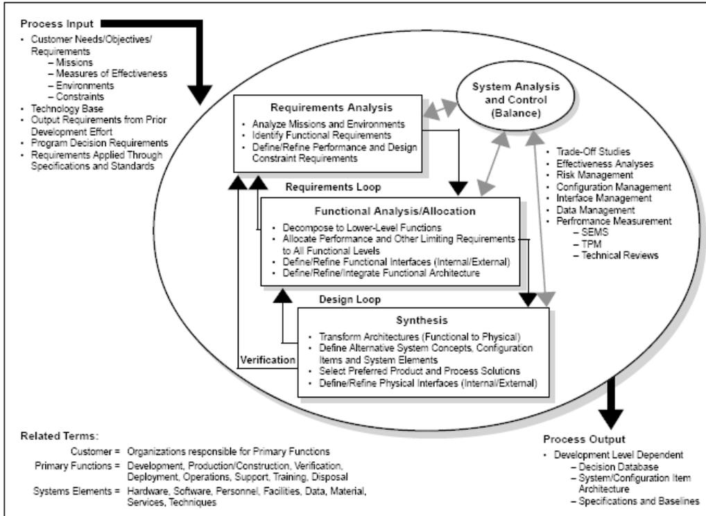
Figure 1. Systems Engineering Process (From DAU, 2001)
