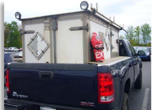
This pickup truck is loaded with a portable magazine designed to meet federal regulations for explosives transportation.
