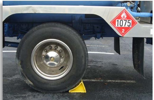
The wheel chock behind the rear axle of this liquefied petroleum gas cargo vehicle is one of several required safety features.
