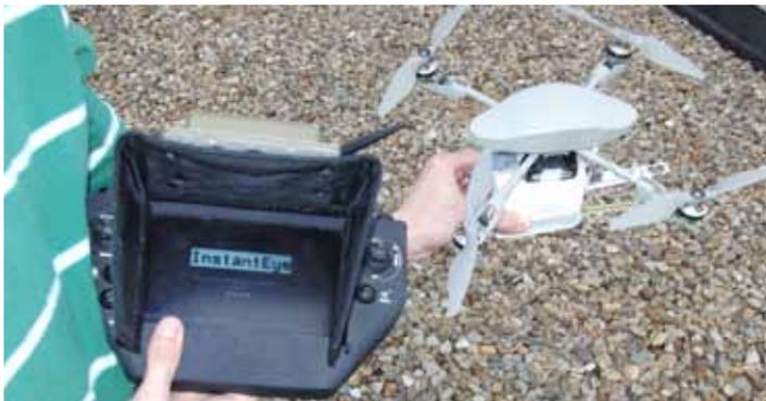
Quad rotor helicopter UAS with controller (left side). The main UAV is grey colored; the person is holding a white radiosonde (a meteorological instrument used to measure air temperature, humidity and pressure) which is attached to the bottom of the UAV. The temperature and relative humidity sensors are in the silver probe extending to the right of the radiosonde.
