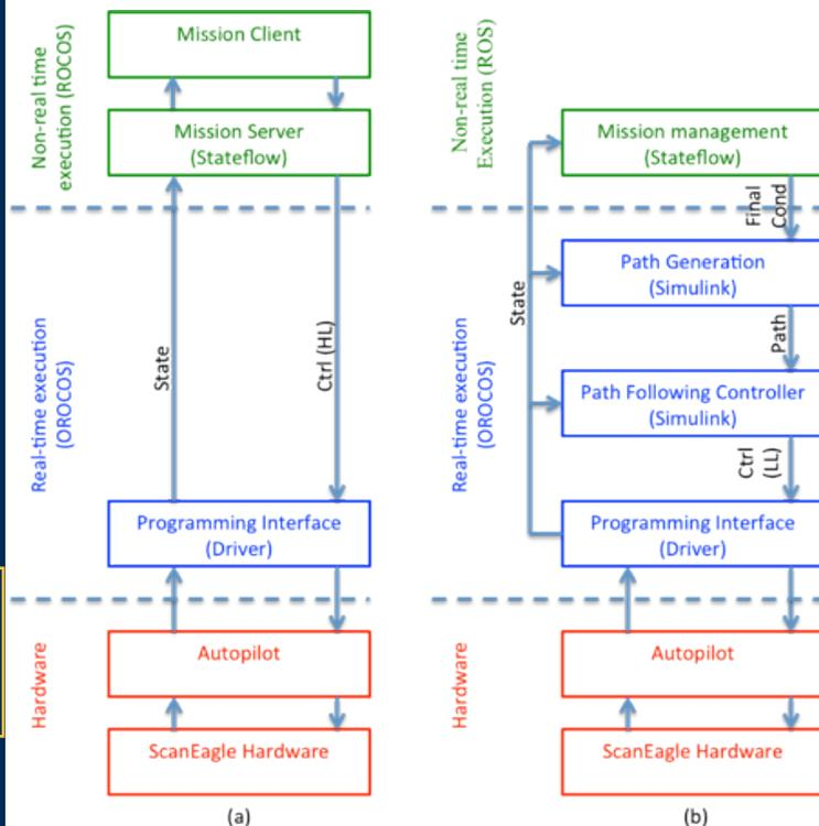
Fig 2: Secondary autopilot architecture for (a) high-level and (b) low-level control interfaces
