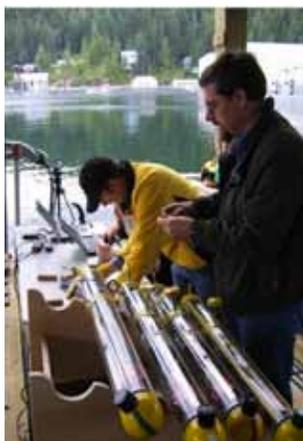
Figure 1. UI mini AUVs being prepared for field testing
