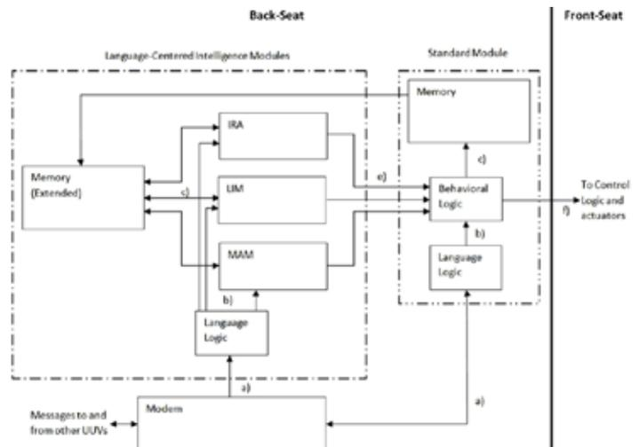
Figure 2. Overall AUV control architecture including LCI module
