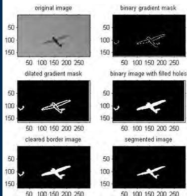
Figure 1. Segmentation an unmanned vehicle from a video frame
