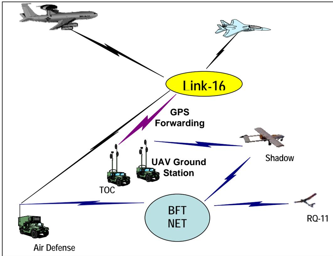
Figure 10. UAV Tracking with Blue Force Tracker
