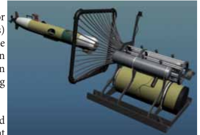
Conceptual picture of the REMUS AUV entering the docking station
