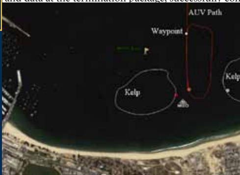
Diagram of preferred AUV approach route for docking relative to the MISO structure (photo courtesy of MBARI)
