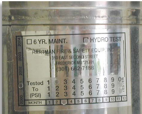
According to the service tag, this stored pressure portable fire extinguisher was pressure tested to 200 psi (1,379 kPa).
