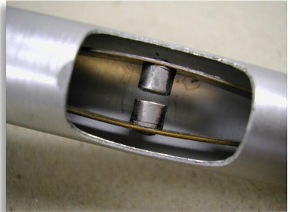
This cutaway closeup of a rate compensated detector shows the position of the electrical contacts in the open circuit position.
