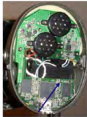
ARM 9 Processor, heart of new integrated translator circuitry, mounted in headset form factor.
