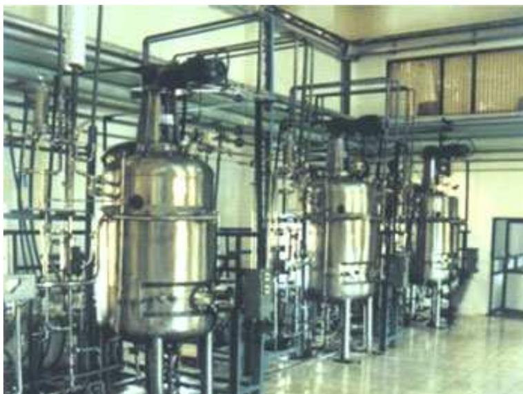
Photo 1: A bank of three Scigenics (India) 1,000 liter fermenters set up to ferment microorganism for enzyme production.
