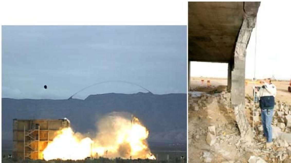
*Figure 9. Testing of structural columns in multi-story office buildings to exterior blast effects.*
