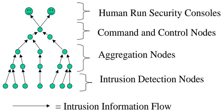
Figure 1: Generic Distributed Hierarchical Intrusion Detection Architecture
